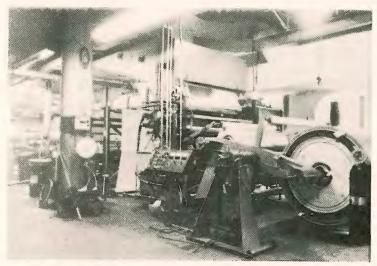
Above, lamination exits the oven stage and is rolled by the final stage of the laminating machine to await trimming.
