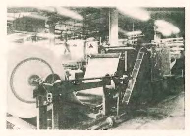
Sheeting machine unrolls completed lamination and cuts it to desired sizes.
