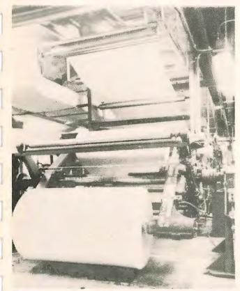
Paper unwind station teeds paper from roll to laminating machine.
